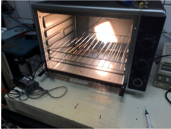
Figure 44: Photograph of the attempt to measure the contact angle by thermalisation. The device was placed in a kitchen oven.
